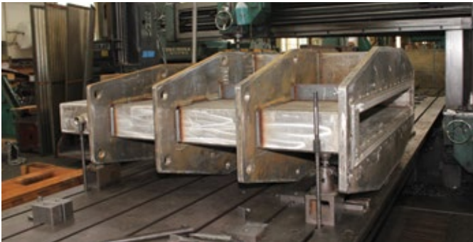
In-House Machining, 72" Bonneted Knife Gate Valve
