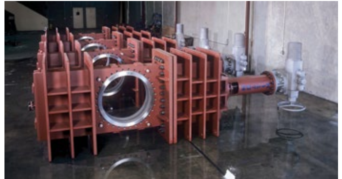
40" Thru-Port Knife Gates, ASME 300, Removable Port Liners, Tungsten Carbide Hardfacing & Abrasion Resistant 410 SS Gate, Abrasive Mine Tailings, Kennecott Copper, Utah
