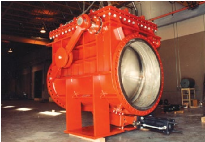
54" Swing Check Valve, Outside Lever & Weight, Bottom Hydraulic Dampener. Wastewater Treatment Plant, Taiwan
