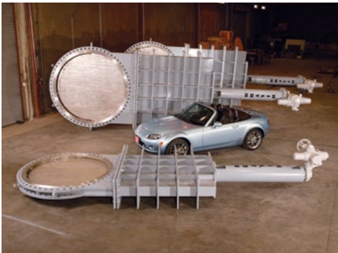
84" & 66" Bonneted Knife Gates, CS Flanges, 304 SS Trim, Electric Motor Actuators, Wastewater Plant, Dallas
