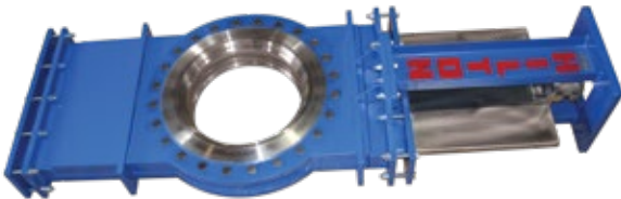
24" Thru-Port Knife Gate, 150 psi, Replaceable Bi-directional Metal Seats, Teflon Internal Cavity Filler, Tianjin Chemical China & GE Plastics Mississippi
